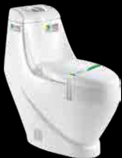
Nancy (C-736) Wash Down One-Piece Closet Size : 675x430x630mm S-trap : 250/300mm, P-trap: 180mm
